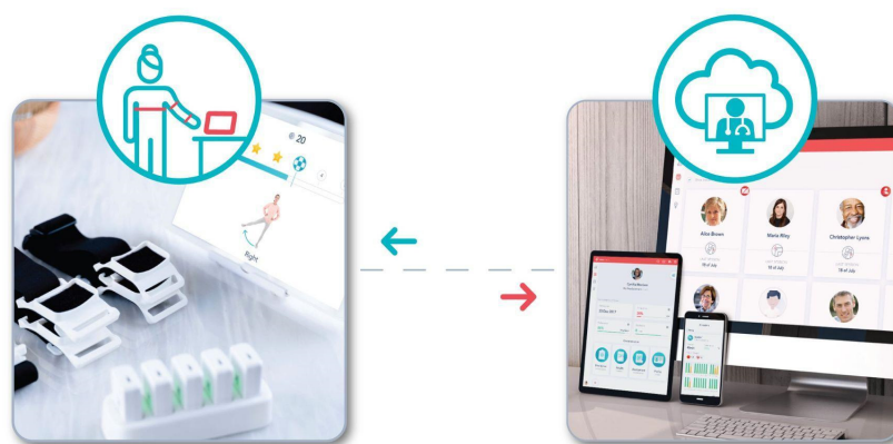
Figure 1. System components. The left figure shows the motion tracker setup and the mobile app displaying the audio-video instructions during the exercise, alongside the real-time biofeedback provided to patients. The right figure depicts the web portal with the results from each patient's session, enabling fully remote asynchronous monitoring by the assigned physical therapist.
