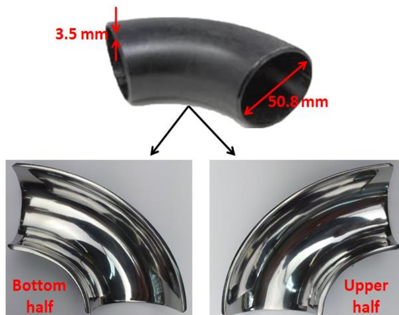
Figure 1. Axially cut sections of a fine polished 90° elbow.
