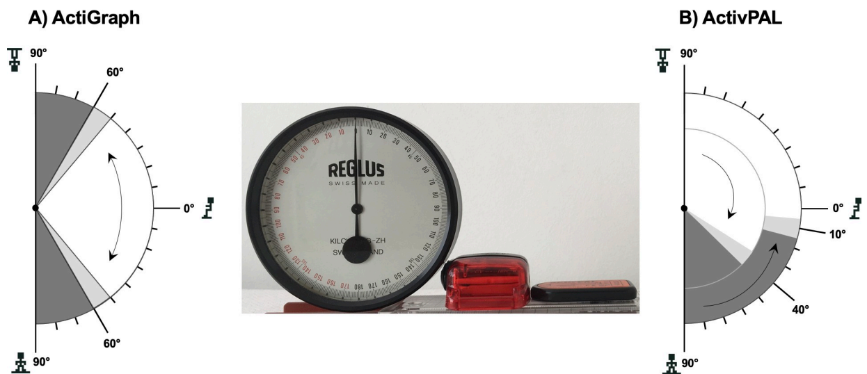
Fig 3. Graphical representation of the results of the angles measurements. Angle measurements for the ActiGraph (3A) and activPAL (3B) using a protractor. The picture in the middle shows the starting position with the devices placed parallel to the floor and the protractor scale reading 0^\circ , representing sitting. The areas in white and grey represent the coded position and angle ranges relative to the horizontal. White = sitting, dark grey = standing, light grey = postural transition (sitting to standing or vice versa). The arrows show the direction in which the devices were moved. The double arrow in 3A shows that the coded position was independent from the direction in which the monitor was moved. The two arrows in 3B highlight differences in the coded posture and postural transition, depending in which direction the monitor was moved.
