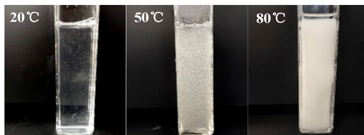
Figure 5. The phase change of thermosensitive hydrogels at different temperatures.
