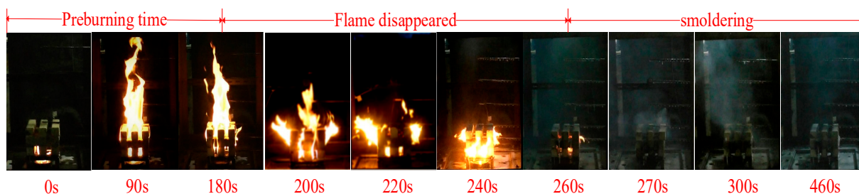
Figure 7. Flame morphology of thermosensitive hydrogel of 6wt% during the fire suppression process.
