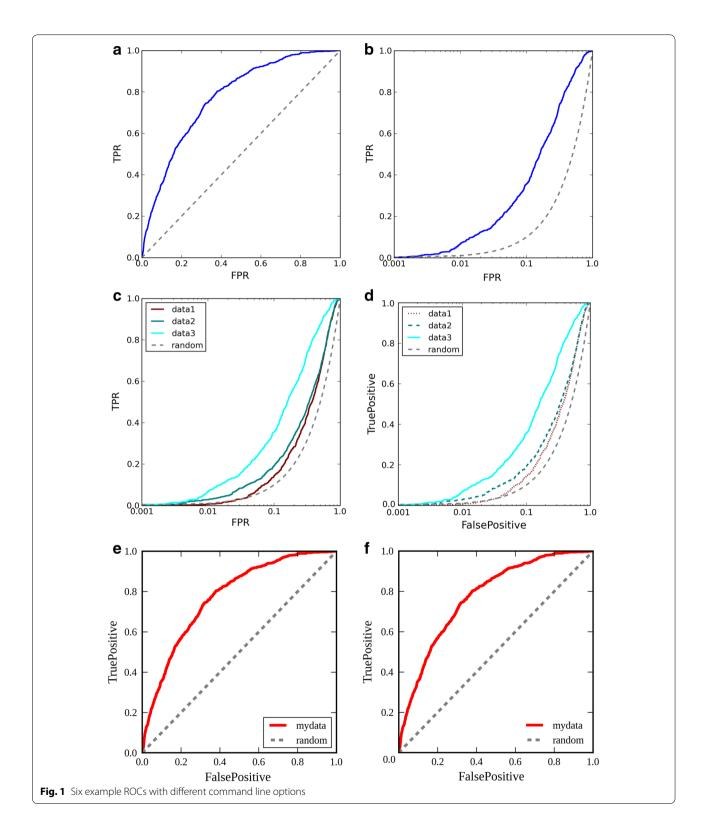
(C) rocker 2.txt 3.txt 5.txt -an CHEMBL -s 5 5 -li data1 data2 data3 random -l 0 -lp 0.001 -cl maroon teal cyan -p Fig1C.png
