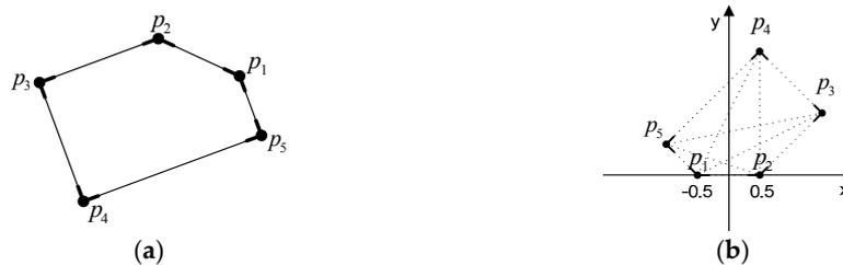
**Figure 5.** (a) Edged corner features derived from a model, and (b) information to be stored in a hashing table (dotted lines represent context features).
