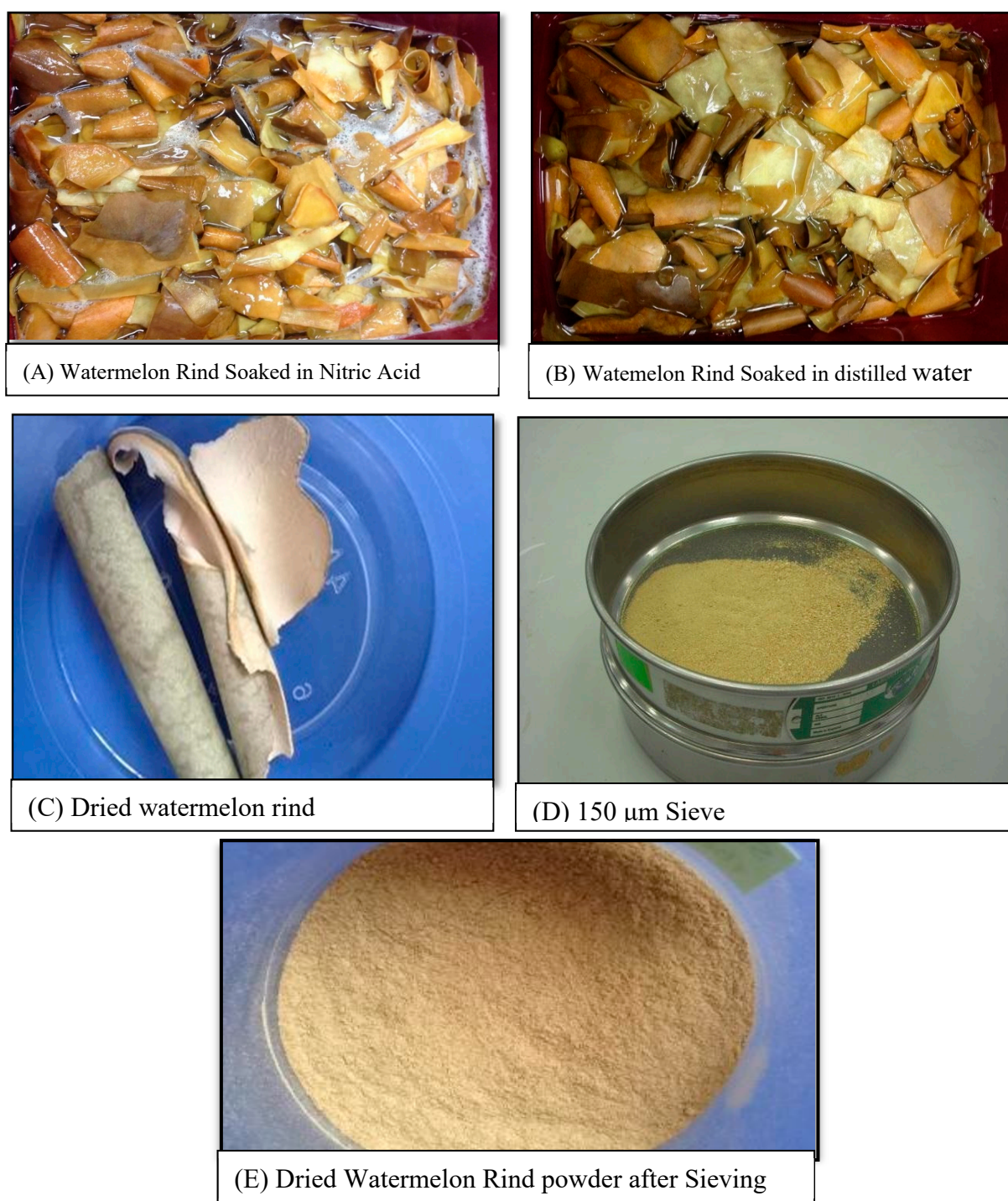
Figure 1. Steps for producing dried watermelon rind powder with 150 \mu\text{m} particle size.
