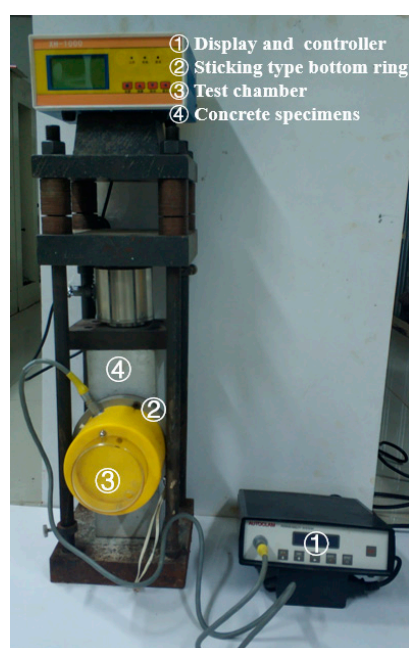
Figure 3. Autoclam test system.
