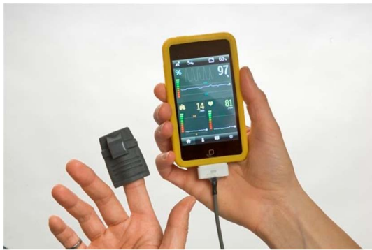
Figure 1. The Phone Oximeter. A mobile device that integrates a pulse oximeter with a smartphone.
