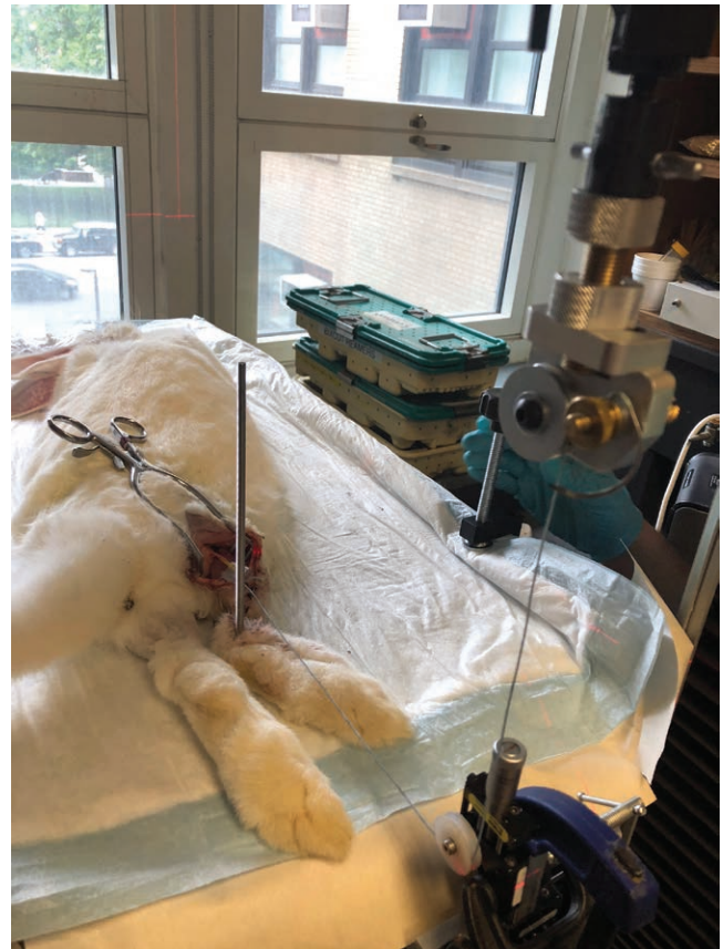
Fig. 3. Experimental setup for assessing pull out strength.
