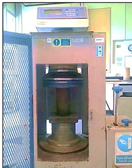
Figure 3. The experimental setup for the ECC compressive test.
