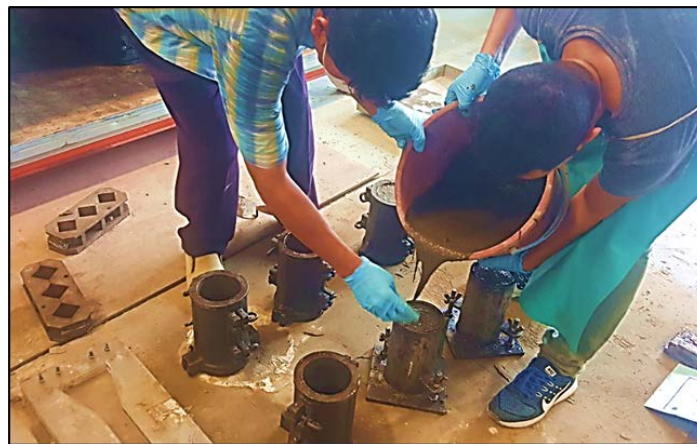
Figure 1. ECC casting on the cylinder molds.
