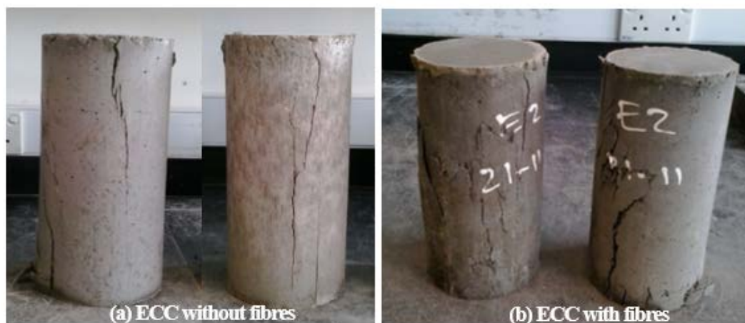
Figure 8. Typical failure condition of ECC samples: (a) for ECC without fibres, (b) for ECC with fibres.
