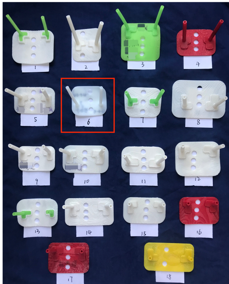
Fig. 3 All of the templates in group A. No. 6 is the deformed template
