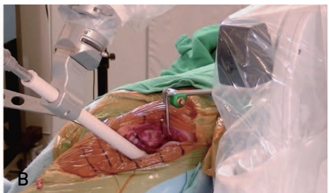
Fig. 8. Robot-assisted total hip arthroplasty for the cup positioning using TSolution One ® system. TCAT ™ is positioned according to the pre-operatively planned orientation of the cup. (A) Schematic drawing and (B) photograph from operation field.
