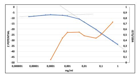
**Figure 10.** I<sub>373</sub>/I<sub>384</sub> intensity ratio obtained from pyrene emission spectra in the presence of poly-6-MOEG-9-T-**BF3k**-FE (blue curve) and Z-potential values (orange curve) as a function of polymer concentration.
