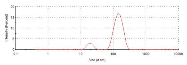
**Figure 11.** DLS size distribution histograms of poly-6-MOEG-9-T-**BF3k**-FE dispersions in ultrapure water.
