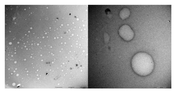
**Figure 12.** Structure of macromolecular aggregates found by TEM analysis of poly-6-MOEG-9-T **BF3k**-FE solutions in water. The scale bar corresponds to 1  $\mu$ m in the left panel and 200 nm in the right panel.
