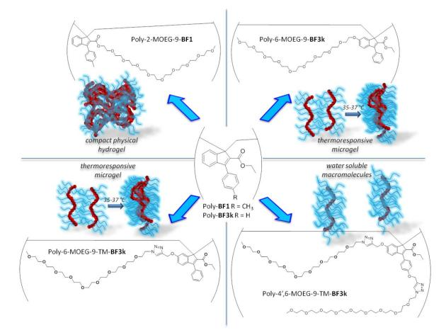
**Figure 1.** The previously proposed aggregation mechanism in PEGylated polybenzofulvene brush (PPBFB) derivatives.
