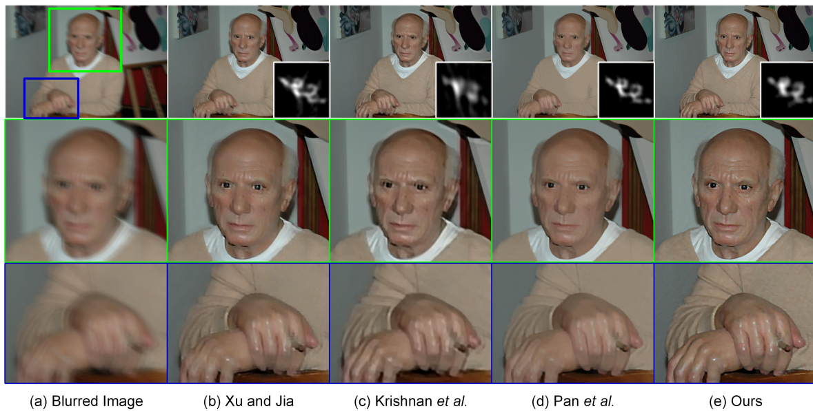
Figure 10. Single-image blind deblurring results with a blur kernel of size 27 \times 27 (top) and their local magnification views (middle and bottom). From left to right: (a) input blurred images, deblurred versions generated by (b) Xu and Jia [11], (c) Krishnan et al. [9], (d) Pan et al. [59] and (e) our proposed method, respectively.
