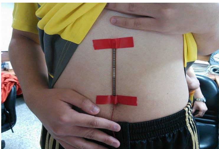
Figure 21. Position for the placement of the wireless respiratory rate detection system.
