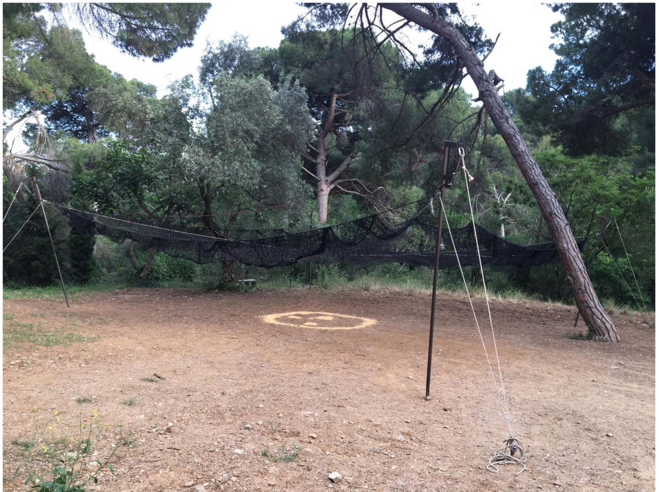
Figure 1. The ESTRATEKO drop-net trap deployed in a peri-urban location of Barcelona city at dusk, ready to run. Corn kernels are used as bait to attract wild boars to the central area under the net.
