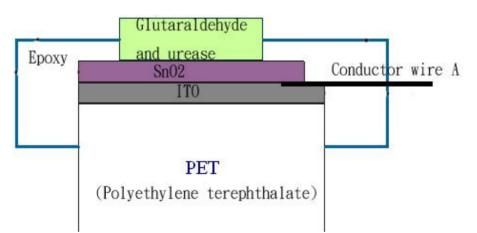
Figure 1. Electrode structure of ion-contact type.
