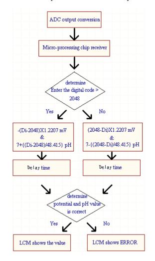
Figure 5. The internal operation of P89C51 for pH measurement.
