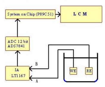
Figure 3. The system structure for potential measurement.
