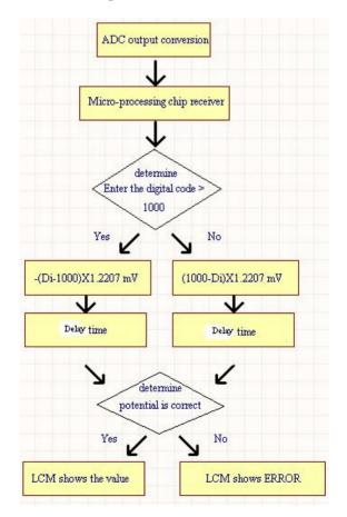
By inputting the microprocessor with the derived code after the electrode was immersed in the PB solution to replace the default code 1000 of ADC, the reset function is attained. It must be noted that the selected IA, ADC and microprocessor chips for the realization of this designed instrument are based on the considerations of appropriate accuracy, low cost and easy modification and debugging for experimental demands.
