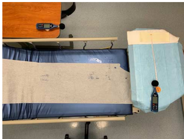
FIGURE 1. Depiction of sound level meters position at 18 and 36 inches relative to testing sample in the closed exam room setting. The sound level meter utilized for the 6-ft measurement is not depicted.
