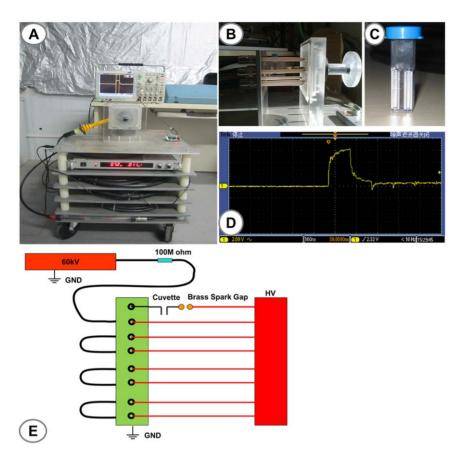
**Figure 1. A schematic diagram of experimental setup for nsPEFs on Cal-27 cells.** A schematic diagram of experimental setup for nsPEFs on Cal-27 cells. A) NsPEF generator; B) Pulse excitation region; C) 0.2 cm gap cuvette (Biosmith); D) The typical waveforms of nsPEFs; E) Circuit design for nsPEFs.
