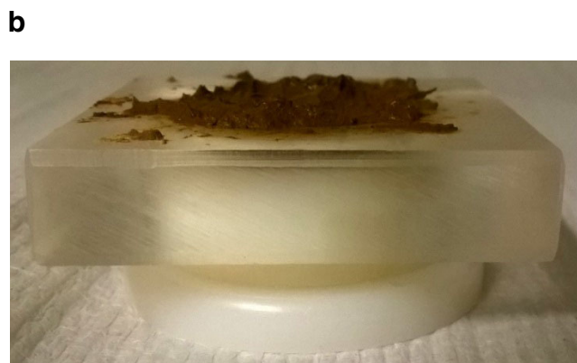
Fig. 1 DGT sampling device schematic (a): 1 piston, 2 outer sleeve with sampling window, 3 resin gel, 4 diffusive gel, 5 protective membrane, 6 plastic frame to hold the soil sample in place, 7 soil sample. Application of the DGT device to soil (b). The figure is taken from [10] following the terms of the Creative Commons Attribution 4.0 International License ( http://creativecommons.org/licenses/by/4.0/ )
