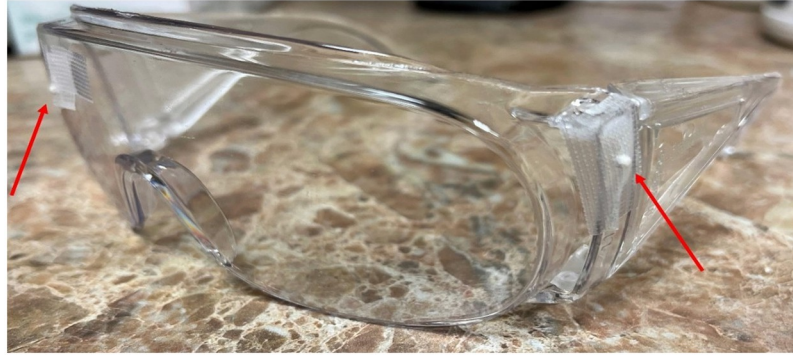
Fig 2. Goggles apparatus. Radiolucent plastic lab goggles worn by the patient with point sources attached to it. Two sources were placed on two sides of the goggles, and one placed on the front near the forehead of the patient. In the figure, two point sources can be seen to be indicated by two red arrows.
