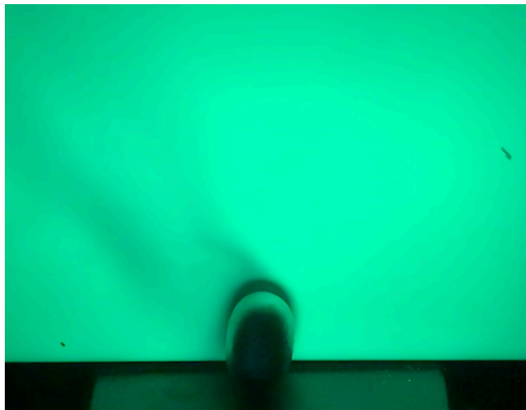
Fig 2. A parad shivling is placed in front of a TLC plate and irradiated with light from a lamp emitting at 254 nm. The light is absorbed by the Hg 0 vapor emitted from the shivling , casting a dark shadow on the fluorescing TLC plate.
