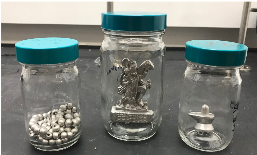
Fig 1. Amalgams can be molded into a variety of shapes including malas (necklaces), deities, and shiva lingams (L→R).
