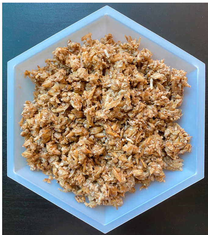
Figure 1. Brewer's spent grain (BSG) consisting of barley malt removed from the lauter tun at the UC Davis Pilot Brewery. Photo courtesy of Emily Newman. Written permission was granted to the authors.
