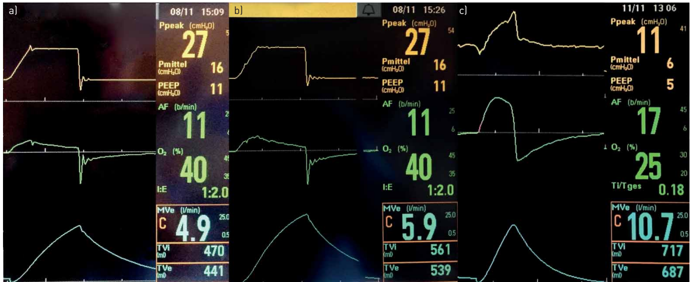
FIGURE 1 Screenshots from the ventilator. Pressure (top, yellow), flow (middle, green) and volume (bottom, blue) curves with corresponding ventilator settings and tidal volume measurements a) immediately before administration of enoximone, b) 15 min after enoximone had been started and c) 3 days later, immediately before extubation. Ppeak: peak inspiratory pressure; Pmittel: mean airway pressure; PEEP: positive end-expiratory pressure; AF: respiratory rate; O 2 : inspiratory oxygen fraction; MVe: expiratory minute volume; TVi: inspiratory tidal volume; TVe: expiratory tidal volume.
