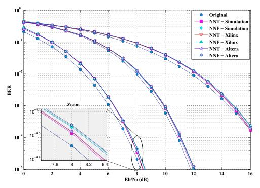
Figure 18. BER of the implementations for a CM1 channel.
