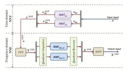
Figure 5. New time-domain and frequency-domain NN for QPSK.
