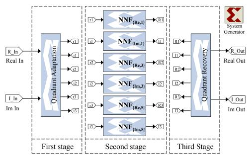
Figure 10. Implemented frequency-domain NN using a Xilinx system generator.
