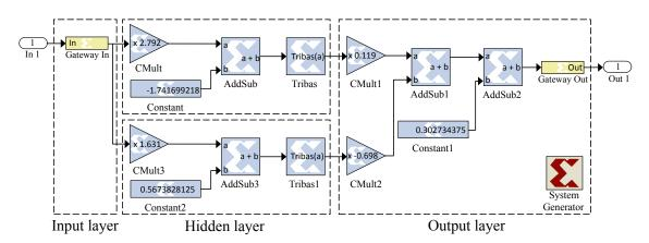
Figure 8. Implemented NN using a Xilinx system generator.
