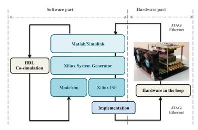
Figure 11. Hardware co-simulation.
