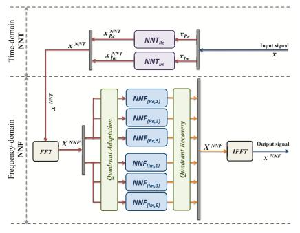
Figure 6. New time-domain and frequency-domain NN for DCM.
