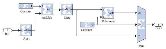
Figure 9. Implemented triangular function using a Xilinx system generator.
