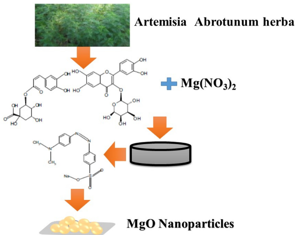
Figure 6. Synthesis of MgO nanoparticles using Artemisia abrotanum Herba Extract. Redrawn from Iranian Journal of Science and Technology, Transactions A: Science, 42, Renata Dobrucka, Synthesis of MgO Nanoparticles Using Artemisia abrotanum Herba Extract and Their Antioxidant and Photocatalytic Properties, 547–555, Copyright (2016), from Springer Nature [144].
