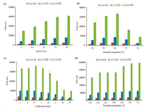
**Figure 5.** Influence of NaCl concentration (**A**), extraction temperature (**B**), extraction time (**C**), and desorption temperature (**D**) on the HS-SPME performance.
