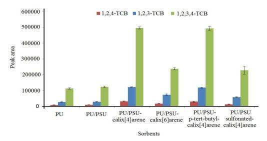
Figure 2. The extraction efficiency of different fabricated nanofibers.
