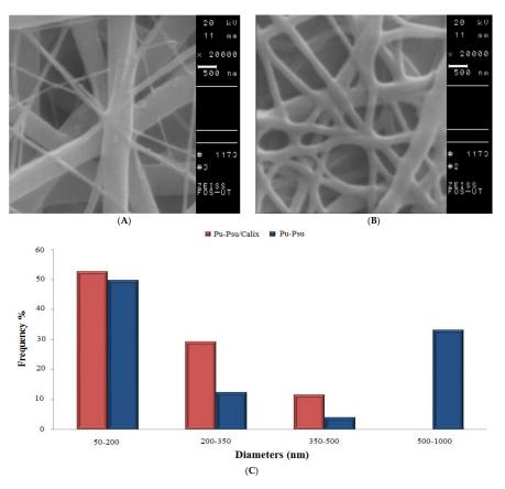
**Figure 4.** SEM micrograph of (**A**) PU–PSU nanofiber, (**B**) calix[4]arene modified PU–PSU nanofiber, and (**C**) fibers diameter histogram.
