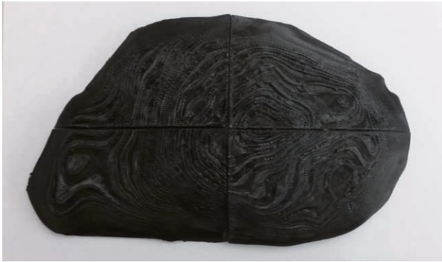
Fig. 7. 3D printed visualization presented to surgeons during the usability interviews. Several models were provided, representing varying levels of smoothing, filling density, colors, and scale. This model was created with the Craftbot XL 3D (CraftUnique, LLC, Stillwater, Okla.) in four sections, which were glued together to demonstrate a printing option with reduced printing time.
