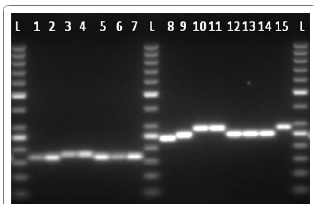
Figure 1 Electrophoretic gel showing VNTR profiles. Lanes 1 to 7 represent the amplification of 7 isolates for marker Asp 330 (11 bp repeat). Samples in lanes 1-2 and 5-7 have 3 repeats and samples in lanes 3-4 have 4 repeats. Lanes 8 to 15 represent the amplification of 8 other isolates for Asp 443 marker (18 bp repeat). Sample in lane 8 has 4 repeats, samples in lanes 9 and 12-14 have 5 repeats, samples in lanes 10-11 and 15 have 7 repeats.
