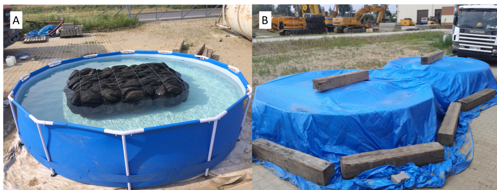
Figure 3 Leachate test trial. (A) Tyre bale in test pool. (B) Test trial protected against atmospheric influences.
