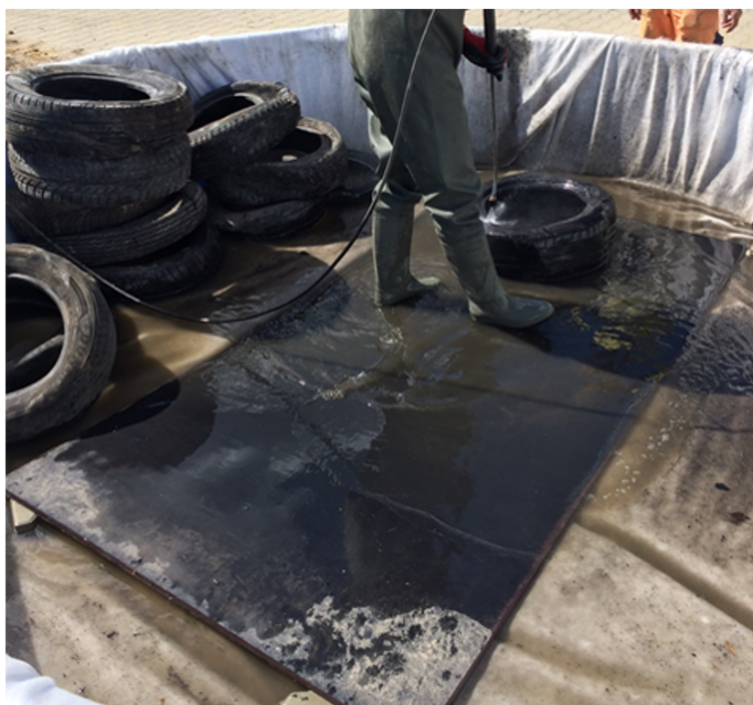
Figure 2 Stage I: washing tyres intended to perform tyre bales; testing leachate.
