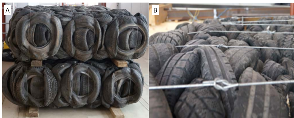
Figure 1 Tyre bales used in research. (A) General view of tyre bale. (B) Detail of connection wires.
