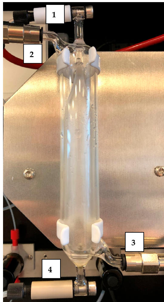
Figure A1. Picture of the scrubber with water inflow at the top (1) and water outflow at the bottom (4). Air inlet is at the bottom (3) and air outlet is at the top (2).
