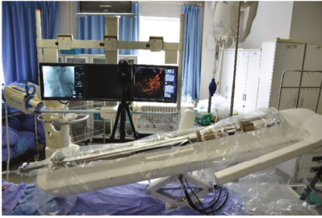
FIGURE 1: The manipulator arm of the slave end.
