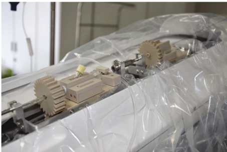
FIGURE 2: The manipulator arm of the slave end holding the guidewire.
