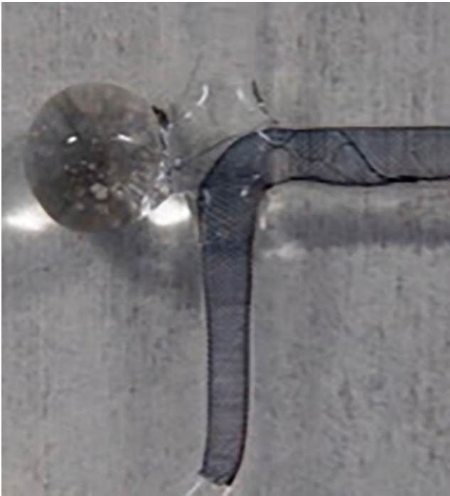
Fig. 3 Glass model of an MCA bifurcation aneurysm showing a pCONUS2 bifurcation device implanted with its petals at the level of the “aneurysmal” neck. A p48MW 2/15 mm is deployed through the pCONUS2 from the “inferior MCA trunk” to the “M1 segment”. There is only a small amount of metal connecting the six petals with the shaft of the p48. This allows the uncompromised expansion of the flow diverter
