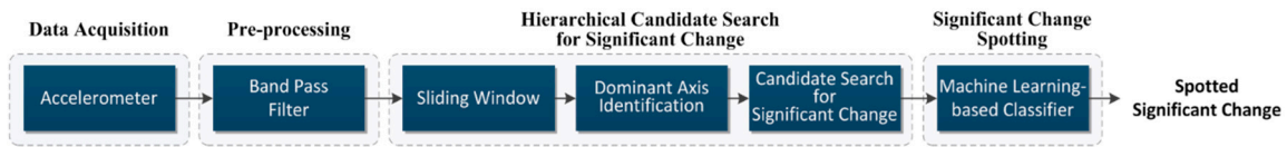
Figure 1. The architecture of the proposed approach for the segmentation mechanism, including data acquisition, pre-processing, hierarchical candidate search for significant change, and significant change spotting.
