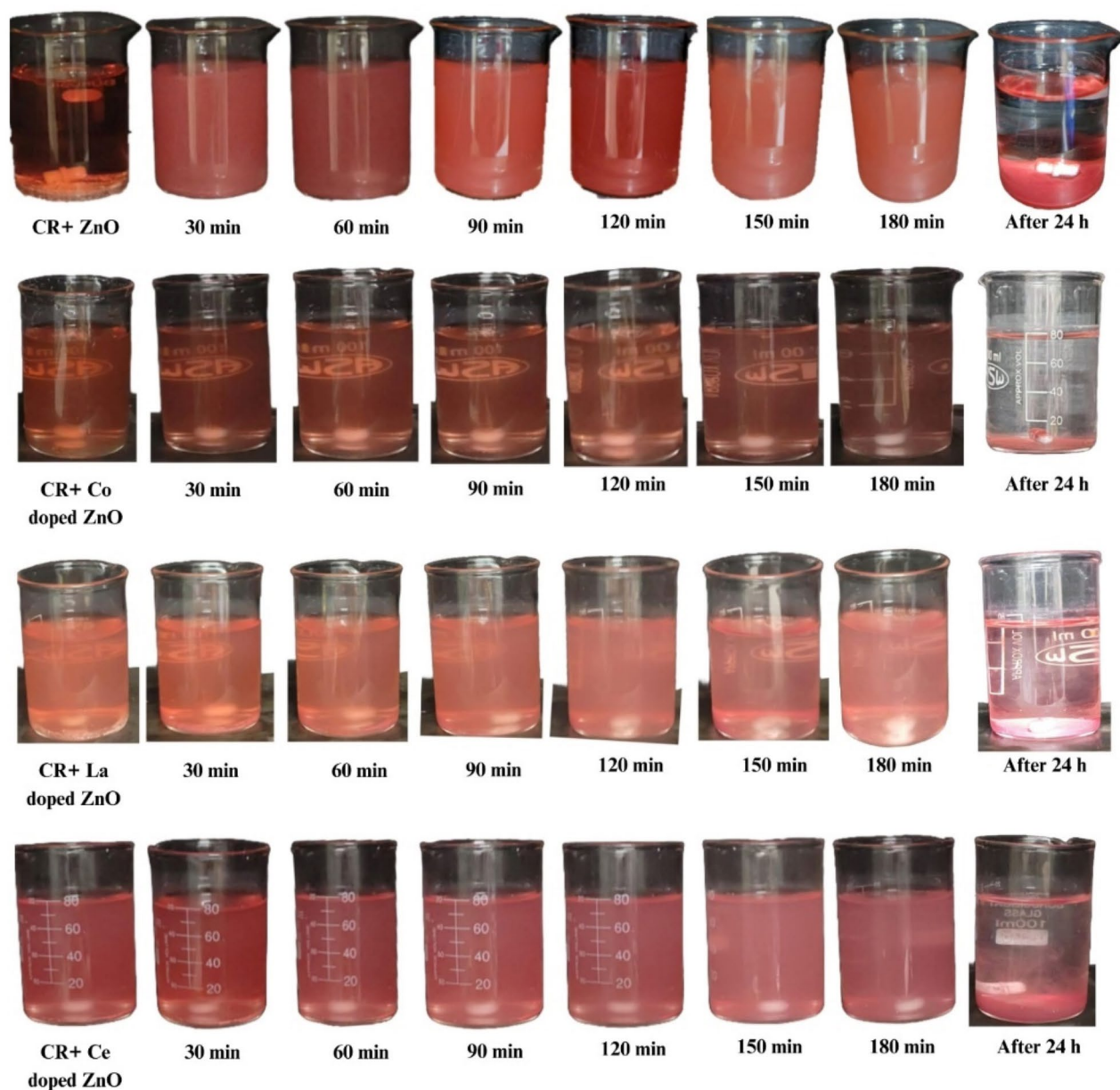
Fig. 20. Pictures of adsorption of CR over ZnO, Co-doped ZnO, La-doped ZnO and Ce-doped ZnO at 30 min intervals until 180 min and then at 24 h period.
