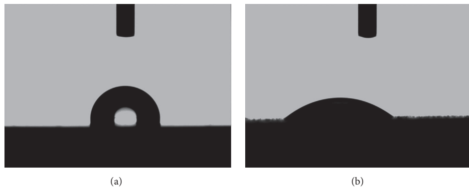
FIGURE 4: Optical images of a water droplet in contact with Co-Cr (a) and TiO 2 (b) surface.
