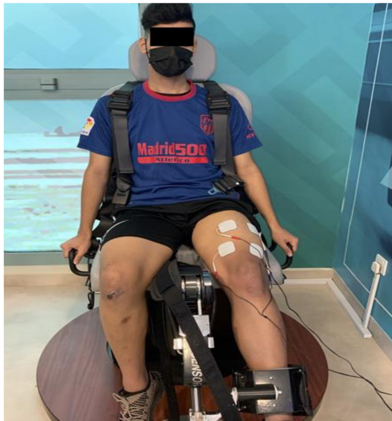
Figure 3 Electrode placement during NMES guided strength training.
