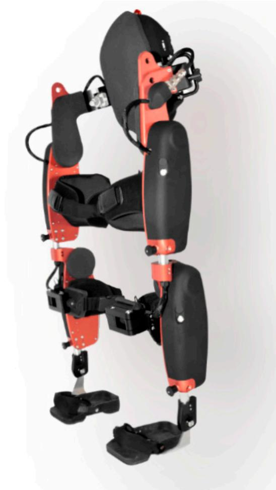
**Figure 1.** Sagittal view of UAN.GO, the exoskeleton used for the present case report. The device is provided of a bilateral four-joint system (hip, knee, ankle and foot), in which proximal joints are computerized (hip and knee), distal ones are fixed (ankle and foot). A central unit allows movement maps execution.
