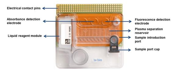
**Figure 2.** The single-use cartridge is comprised of a printed circuit board and a plastic top plate. Notable features include the sealed liquid reagent module, sample loading port, and dried reagents (not shown).
