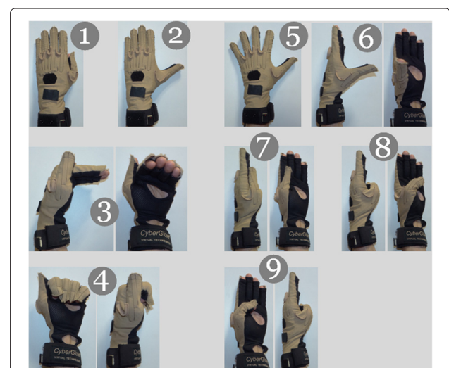
Figure 2 Key-postures that every subject had to perform once during the calibration phase. This phase was performed once by each subject prior to the grasping tasks and the calibration obtained was then used during the entire experimental session.
