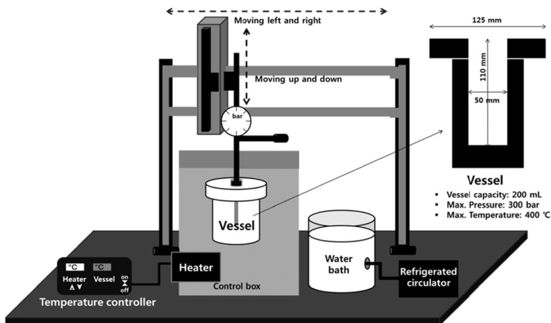
Fig. 1. Schematic diagram of Super-H<sub>2</sub>O or Sub-H<sub>2</sub>O system.
