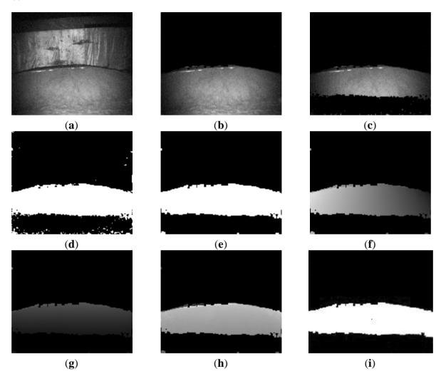
**Figure 14.** The obstacle detection process and results of proposed method in Scene 5. (a) Original image (b) Far background removed (c) Ground and sky region removed; (d) Binary image of ROI (e) Image erosion and dilation (f) Horizontal information of scene; (g) Height information of scene (h) Depth information of scene (i) Detected obstacles.
