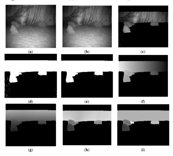
**Figure 11.** Obstacle detection process and results of proposed method in Scene 2. (a) Original image (b) Irrelevant region removed (c) Binary image of ROI; (d) Image erosion and dilation (e) Z dimension information of scene (f) Detected obstacles.
