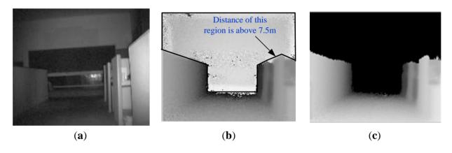
**Figure 5.** "Back folding" measurement filtering in ditch scene based on proposed method [65]. (a) Gray image of ditch scene c (b) Depth image of ditch scene (c) Depth image after processing.
