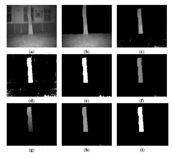
**Figure 13.** Obstacle detection process and results of proposed method in Scene 4. (a) Original image (b) Far background removed (c) Ground and sky region removed; (d) Binary image of ROI (e) Image erosion and dilation (f) X dimension information of scene; (g) Y dimension information of scene (h) Z dimension information of scene (i) Detected obstacles.
