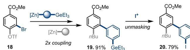
**Scheme 3.** Compatibility of germylated organozinc in cross-coupling and unmasking by iodination. Reaction conditions: a) **1** (2.5 mol%), **18** (0.2 mmol), RZnCl (0.3 mmol), toluene (2 mL), argon, r.t., 5 min. b) **1** (2.5 mol%), ArOTf (0.2 mmol), *n*BuZnCl·LiCl (0.3 mmol), NMP (2 mL), argon, r.t., 10 min. c) **19** (0.18 mmol), DMF (1.8 mL), NIS (0.36 mmol), 60 °C, 30 h.
