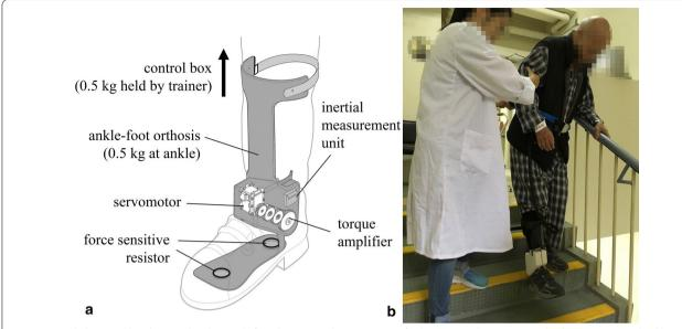
Fig. 1 a Exoskeleton ankle robot used in this study for robot-assisted stair training of sub-acute stroke survivors in both power-assisted ankle robot (PAAR) group and swing-controlled ankle robot (SCAR) group. b Robot-assisted stair training
