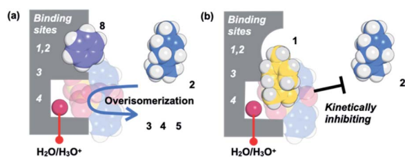
Fig. 7 A possible mechanism that kinetically suppresses over-isomerization inside the MMF by sterically blocking the acid sites that are housed deep inside.
