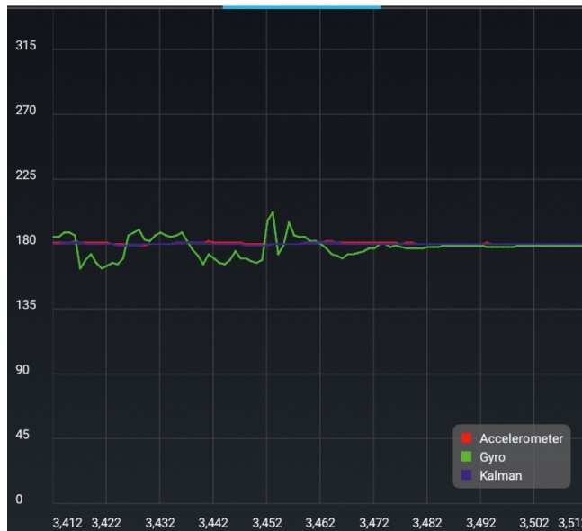
FIGURE 14: Acceleration, rotation angular velocity, and filtering curve.
