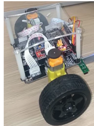
FIGURE 11: Two-wheel self-balancing vehicle system.
