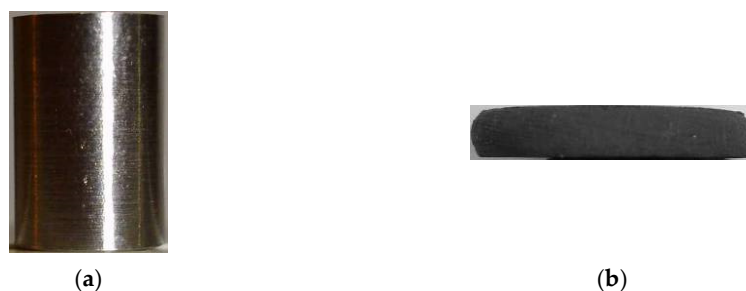
Figure 3. Compression specimen morphology: (a) Before deformation; (b) after deformation.
