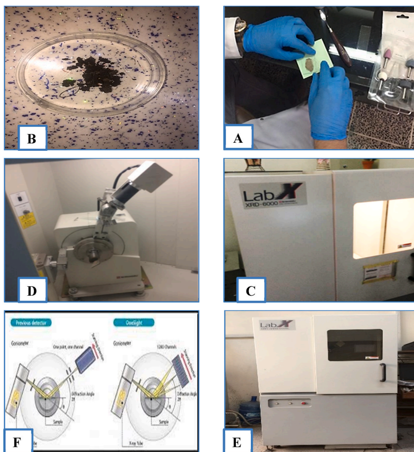
Figure (3). Photographs of the equipment used for the sample preparation for X-ray diffraction research (A) and (B), Shimadzu X-Diffractometer (XRD-6000).
