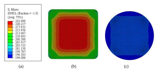
**Figure 12.** Stress contour diagram of central region with two type specimens. (**a**) stress contour bar; (**b**) original specimen; and, (**c**) optimum specimen.
