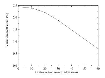
Figure 6. Effect of central region corner radius on stress in central region.
