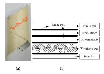
Figure 1. Envelope material [18], (a) macro morphology; (b) Typical envelope material.
