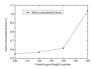
Figure 5. Effect of central region length on stress concentration factor.
