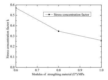
Figure 9. Effect of modulus of strengthening material on stress concentration factor.
