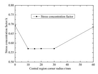
Figure 7. Effect of central region corner radius on stress concentration factor.
