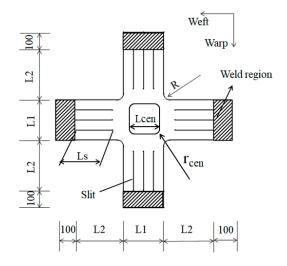
Figure 3. Geometry of modified cruciform specimen (Units: mm).
