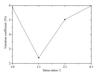
Figure 10. Effect of stress ratios on stress in central region.
