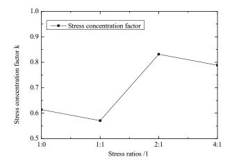
Figure 11. Effect of stress ratios on stress concentration factor.
