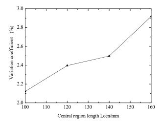
Figure 4. Effect of central region length on stress in central region.
