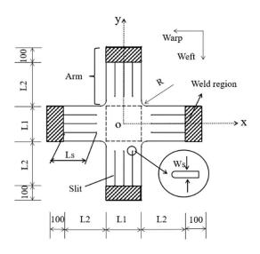
Figure 2. Geometry of base cruciform specimen (Units: mm).
